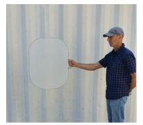
The picture on the left is an example of a good setting – the picture is taken from the point of view of the MetCam. There is a metallic man-made item in the background that is hotter than the ambient air and the ST is fully seen by MetCam.
